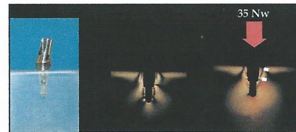
Photoelastic analysis of a Xsign sample.
