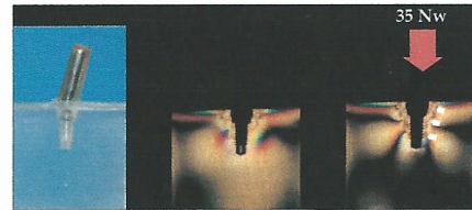
Photoelastic analysis of a SSO sample.
